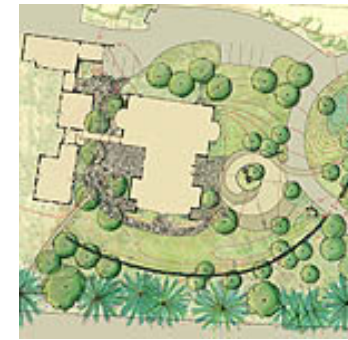
Site plan showing the approach, field stone wall, and retention ponds. Image: Hines Wasser & Associates LLC.
